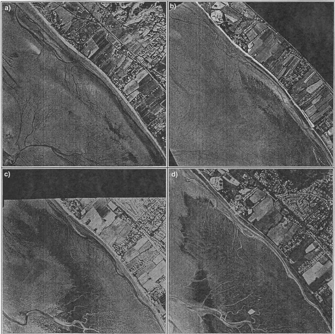
FIG. 3. Historical sequence of black and white aerial photographic images of Area 1 near Heswall: (a) 1955, (b) 1965, (c) 1975, (d) 1997. Dark areas indicate unanalysed areas not included in photographic coverage (Scale 1:16000).
