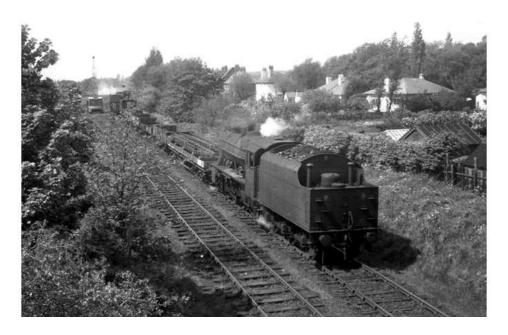
A Stanier-designed 8F 2-8-0 loco is in charge of one of the demolition trains on the stretch of line between Station Road and Moorside Lane. The houses to the right are in Parkgate Road. The track in the foreground is the former branch to Neston Colliery. The loco is one of a large class that latterly were the mainstay of London Midland freight work, surviving until the end of British Railways steam haulage in 1968; about a dozen were based at Birkenhead.
